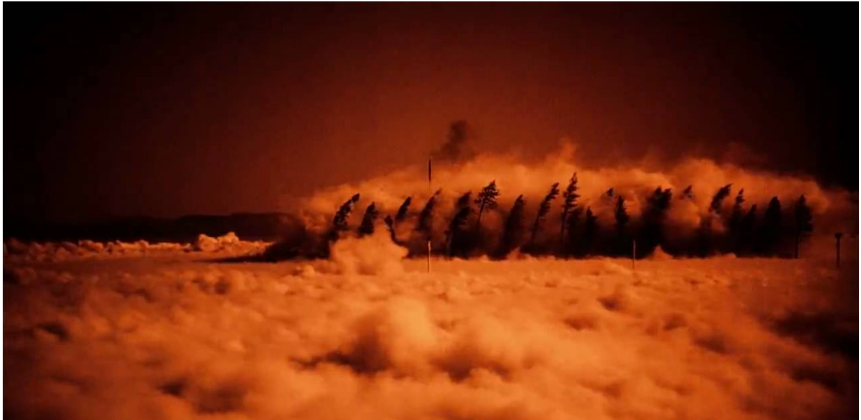
The coniferous tree stand in the Encore test on May 8, 1953. The Atomic Energy Commission had worked with the USDA Forest Service to acquire 145 ponderosa pines from the nearby national forest. The US Army cemented each tree trunk into a concrete block so they would stand upright. Photo courtesy the National Nuclear Security Administration /Nevada Site Office.
